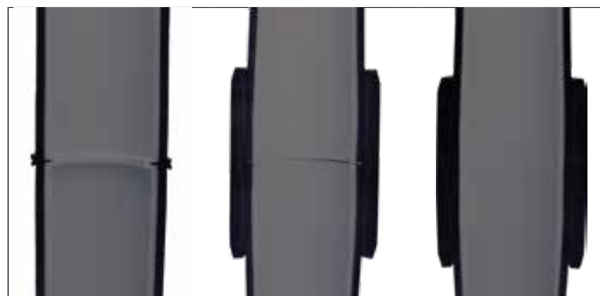
Heated element butt welding
